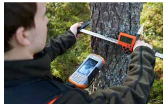
Efficient fieldwork with the MD II caliper used to measure and register tree diameters with direct transfer of results to handheld computer for extended data storing and processing capacities.
